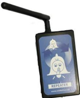
The **repeater** is a standalone unit that is placed between the Transmitter and Receiver and will take the signal from the transmitters and repeat it thus extending the range and removing "blind" spots.
