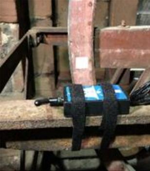
The reflectors that are provided with your transmitter are self-adhesive, however you will need to give them a decent surface to adhere to, clean the area you are going to place the sensor with an alcohol based cleaner (spectacle cleaning wipes are great for this) and then peel off the backing and stick the reflector onto the wheel.
