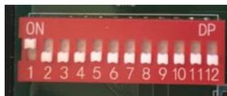
**Note:** Ensure that you power the unit off and on after changing a switch and disconnect the receiver from USB to ensure the channel is changed
