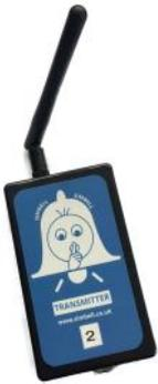
The **transmitter** is installed onto the bell frame and is used to detect the position of the bell wheel using a self adhesive reflector that is placed on the bell wheel to indicate the position of Bottom Dead Centre (BDC) of the bell.
