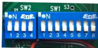
**Note:** Ensure that you power the unit off and on after changing a switch and disconnect the receiver from USB to ensure the channel is changed
